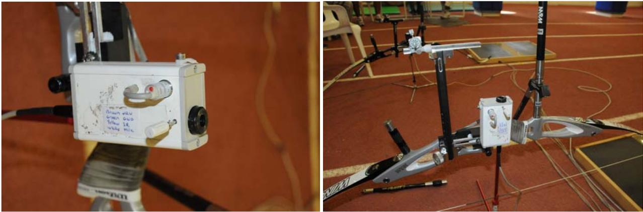
**Picture 2. Detector of clicker drop sound and infrared beamer box attached on a bow.**
